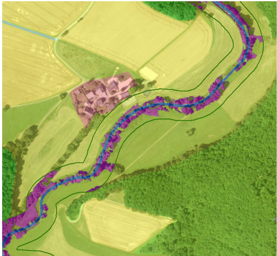
Fig. 3 Example of an orthophoto overimposed to a land cover dataset. In dark blue, the river line. The dark green line defines the buffer area 30 m at each side of the river. In purple, the areas identified as riparian woody features
