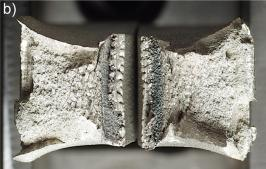
**Figure 17.** Fractures of Charpy test EOS M 290 specimens presented as: (a) fractured Charpy EOS M 290 specimens; (b) fracture surface (optical microscope image) of the EOS M 290 316L, specimen 436. The samples have been numbered, which are visible in the figure. The letters L and R stand for the left-hand and right-hand sides of the sample in the figure. A green check mark means the specimen whose fracture faces were shown.
