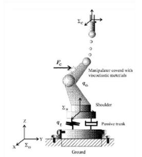
The goal of this cover is to lessen impact forces while keeping contact. Viscoelastic coatings are also used as a suitable component for contact force reduction in [9], along with a deformable trunk consisting of springs and dampers, which is located between a fixed base and the robotic arm.
