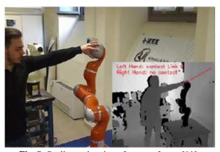
Fig. 8. On-line estimation of contact forces [11].
