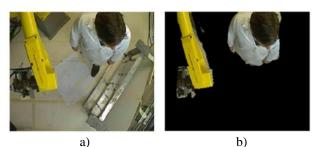
**Fig. 10.** Foreground segmentation in colour images based on foreground detection of 3D points in [15]. (a) Original image. (b) Foreground segmentation in the colour image.
