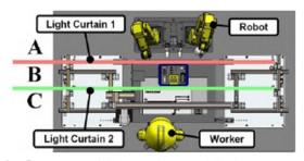
**Fig. 5.** Scheme of light curtains establishing three safety working areas in a cellular manufacturing operation, [12].
