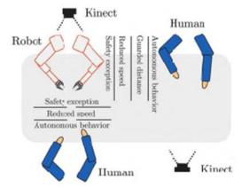
**Fig. 6.** Different robot behaviours in the experimental set-up for multiple HRC using RGB-D devices, [13].
