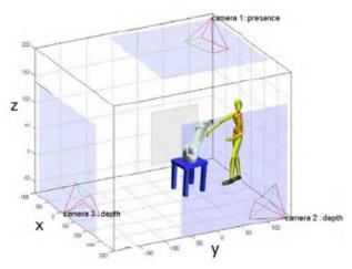
**Fig. 9.** A presence sensor and two depth sensors in their optimal [14].
